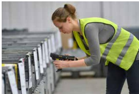
is the ability to verify actions and products by using a bar code scan. Actions, generally termed 'movements' in a WMS, can be scan-verified to provide a check on correct execution. For example if an operative is instructed to place a pallet in a given space, a barcoded location label can be scanned to confirm the location is correct, trapping a potential placement error at source.
